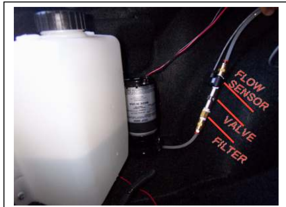
FIGURE C: Pump, Tank and flow sensor installed.
