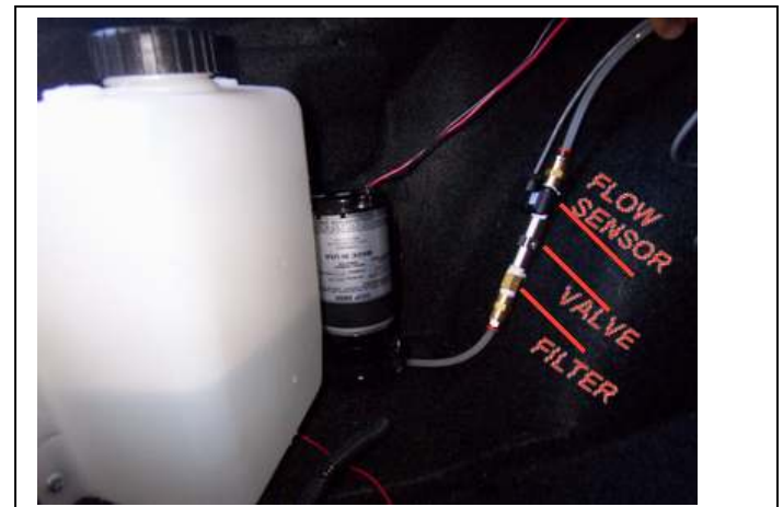
FIGURE C: Pump, Tank and flow sensor installed for trunk install.
