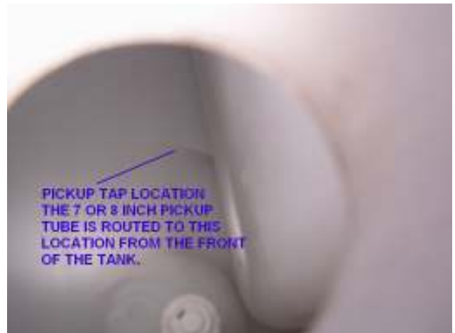
FIGURE E: View of trunkmount tank from under the lid. Tank pickup tube routing.
